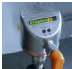
Field-mount monitors can be direct mounted or remote mounted.
